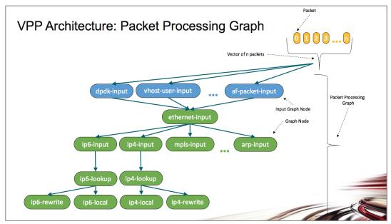
Figure 2. VPP Architecture: Packet Processing Graph of Nodes.
