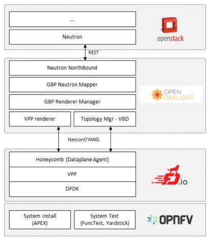
Figure 4. OPNFV FastDataStacks Components.
