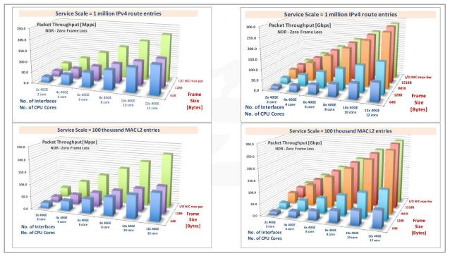
Figure 7. FD.io VPP Data Plane Forwarding Performance – Speedup with Multi-core Multi-threading.
